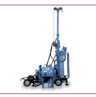
**Lowering trolley.** For moving the drilling around a working site.
