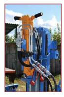
**Hydrohummer** is intended for lowering sampling rods with diameter 121 mm to collect undisturbed samples at geotechnical investigations.
