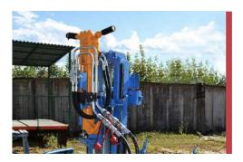
**Hydrohummer** is intended for lowering sampling rods with diameter 121 mm to collect undisturbed samples at geotechnical investigations.
