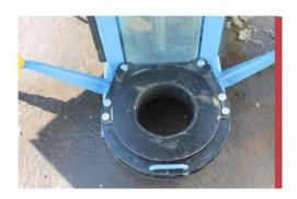
**Casing centralizer.** For drill rods, casing pipes centration at drilling.
