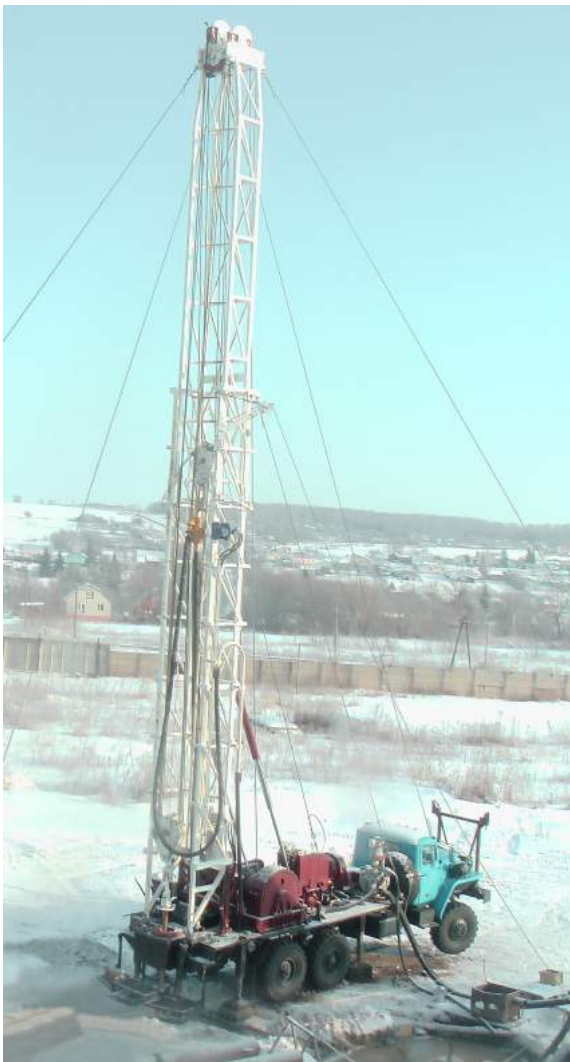
Drilling rig URB-40 onto the URAL-4320 chassis
