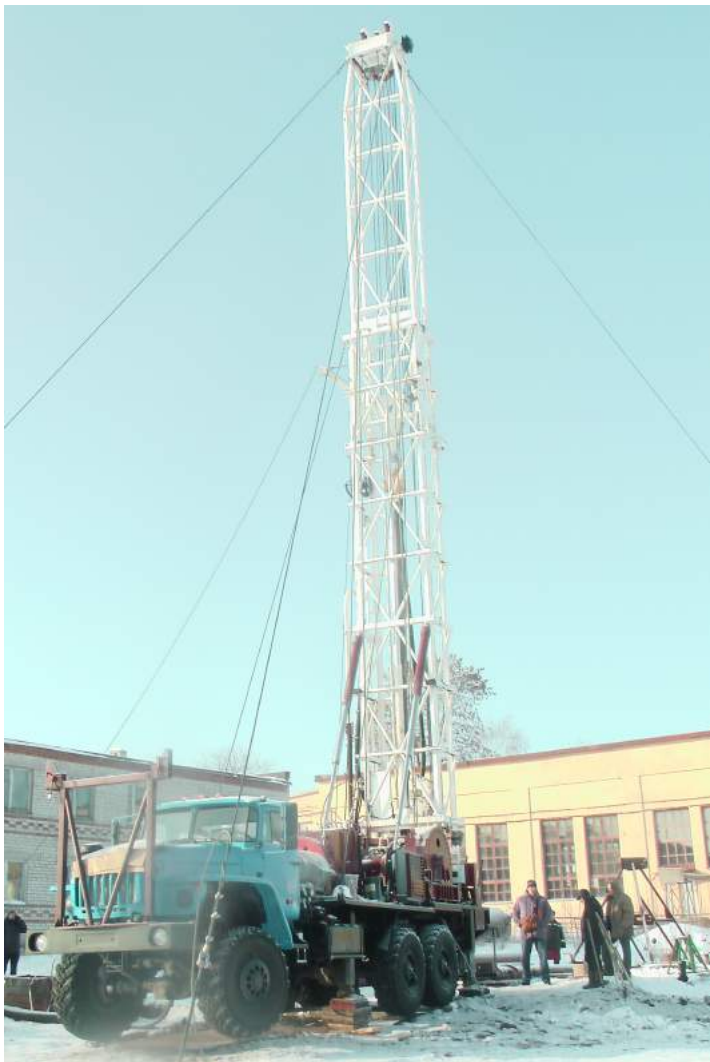
Drilling rig URB-40 onto the URAL-4320 chassis
