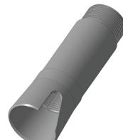
**Cone Catch** - It is used for extraction of emergency drill pipes for the external threads cut by it on a pipe or lock (according to GOST 8565-81).
