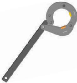
**Key bounce** is designed for initial unscrewing (straining) of tightened threaded nipple and lock joints of the drill pipes.
