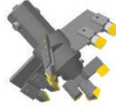
With changeable flat cutters R-35, tops of the blades are reinforced by hard alloy teeth (octagon) D=420,530 mm.
