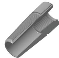
**The fishing tap** - is used for extraction of emergency coring, casing pipe for an internal thread on a pipe according to (GOST 8565-81).
